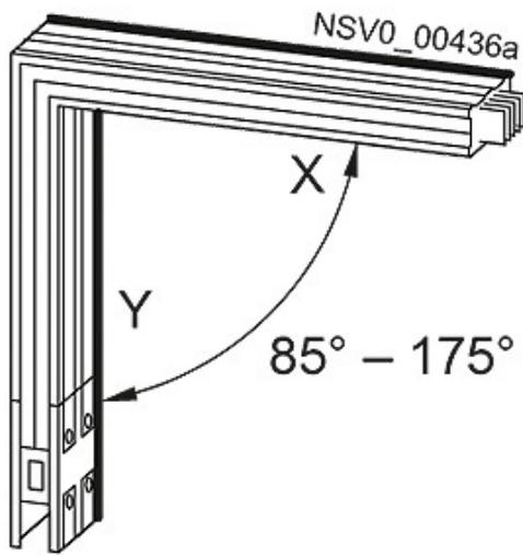
BD2A-400-LH-Y\*-G\* KNIE HINTEN X 0,36M / Y 0,36M-1 ,25M 160A-400A WINKEL 85 GRAD-1 75 GRAD
