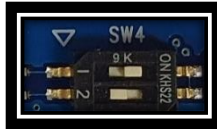
Figure 9: SW4 Set to Use Bluetooth® LE RF Path
