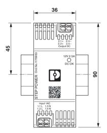
Figure 6 Device dimensions (dimensions in mm)
