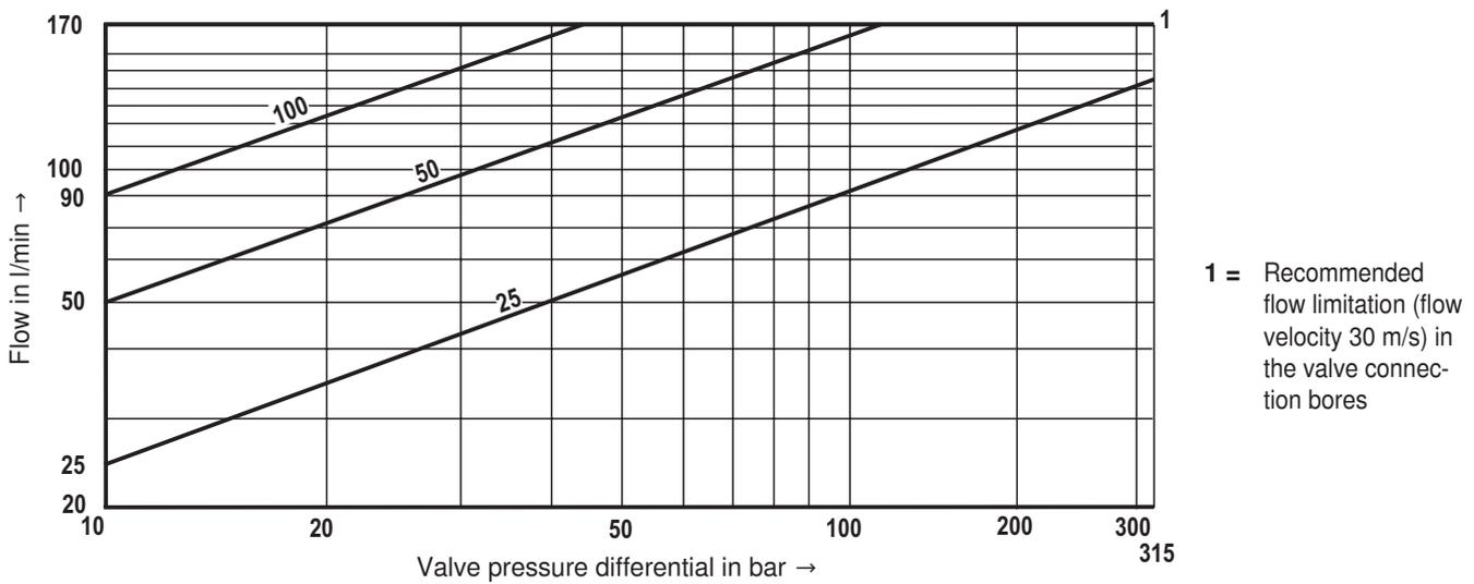
**Characteristic curves: Size 16 (measured with HLP46,  $\vartheta_{oil} = 40 \text{ }^\circ\text{C} \pm 5 \text{ }^\circ\text{C}$ )**
