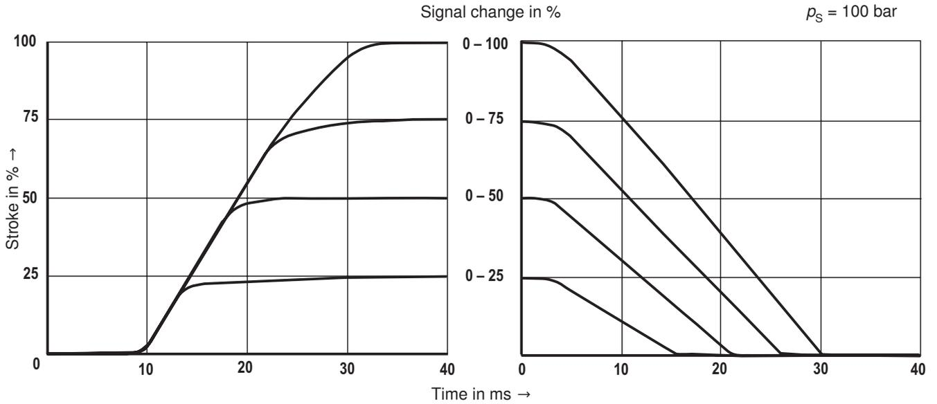
**Flow/load function with maximum valve opening**
