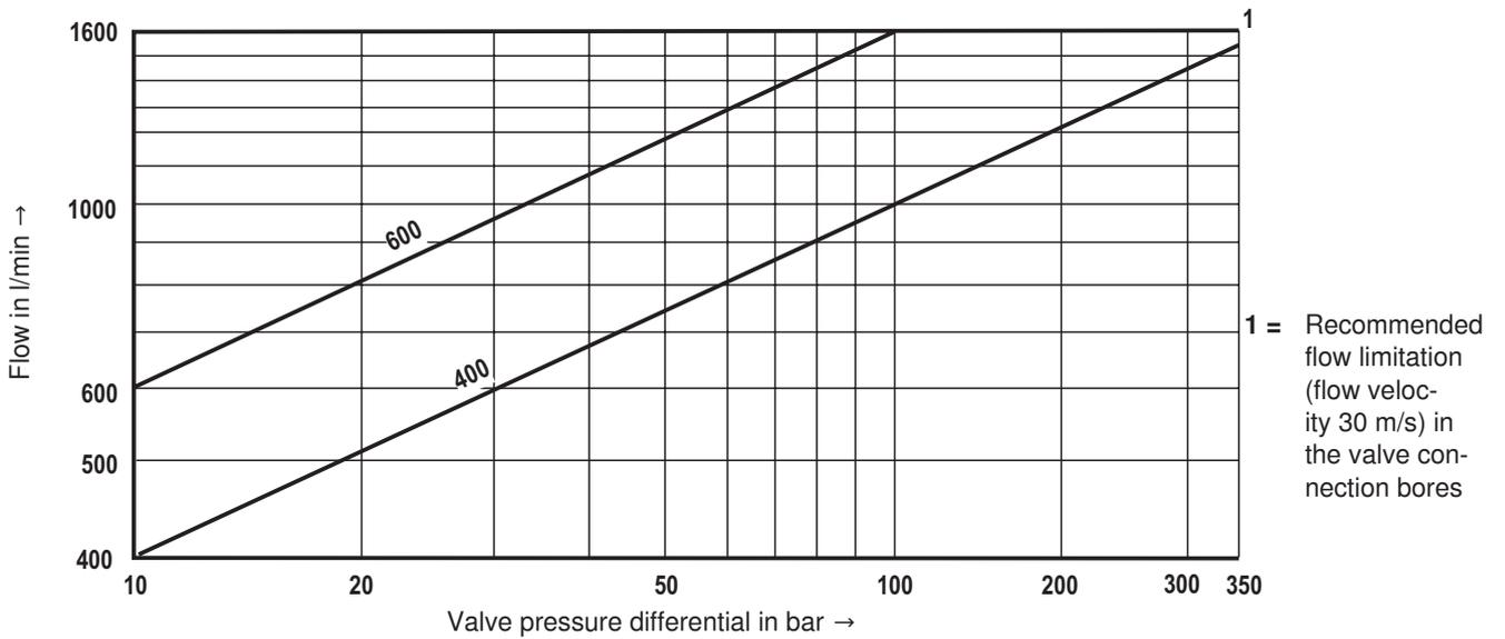
**Characteristic curves: Size 35 (measured with HLP46,  $\vartheta_{oil} = 40 \text{ }^\circ\text{C} \pm 5 \text{ }^\circ\text{C}$ )**
