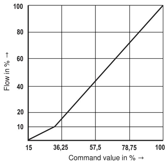
**Characteristic curves: Size 10 (measured with HLP46,  $\vartheta_{oil} = 40\text{ °C} \pm 5\text{ °C}$ )**
