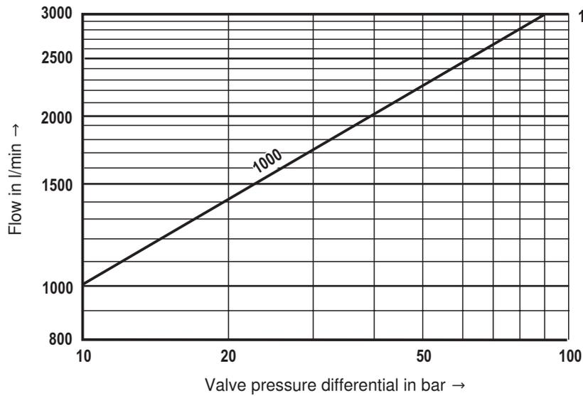
**1** = Recommended flow limitation (flow velocity 30 m/s) in the valve connection bores
