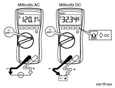
With the function switch in the  $m \widetilde{v}$  position, the Meter measures ac plus dc millivolts. Press to switch the Meter to dc millivolts.
