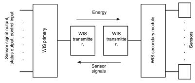
The sum of the currents of all sensors attached to the WIS secondary module must not be greater than the maximum transferable current. This is calculated by dividing the transferable power by the 12 V provided by the transmitters.
