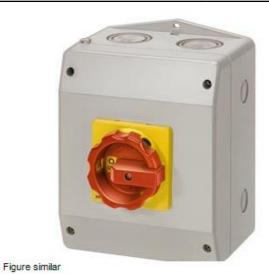
EMERG. STOP SWITCH 6-POLE IU=25, P/AC-23A AT 400V=9.5KW 1NO+1NC, 1 N-TERMINAL INSULATION-ENCLOSED, IP65 ROTARY ACTUATOR RED/YELLOW (EMERG. STOP)
