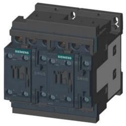
REV. COMB., AC3, 18.5KW/ 400V AC110V, 50/60HZ, 3-POLE, SZ S0 SCREW TERMINAL ELECTR. AND MECH. INTERLOCK 2NO INTEGR.
