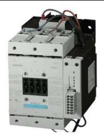
CONTACTOR, 55KW/400V/AC-3 AC(40...60HZ)/DC OPERATION UC 200...277V AUXIL. CONTACTS 1NO+1NC 3-POLE, SIZE S6 WITH BOX TERMINALS ELECTRONIC OPERATING MECHANISM WITH PLC/SIMOCODE INTERFACE AND REMAIN. LIFETIME INDICATOR
