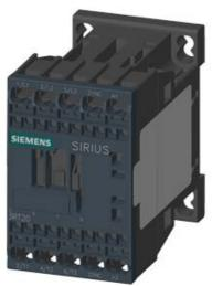
CONTACTOR, AC-3, 7.5KW/400V, 1NC, AC 230V, 50/60 HZ, 3-POLE, SZ S00 SPRING-LOADED TERMINAL
