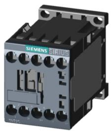
2NO+2NC CONTACTOR, AC3: 4KW DC 110V 50HZ, 120V 60HZ 4-POLE, 2NO+2NC, SZ: S00, SCREW TERMINAL
