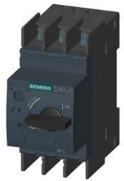
CIRCUIT-BREAKER SZ S00, FOR MOTOR PROTECTION, CLASS 10, A-REL. 0.45...0.63A, N-RELEASE8.2A RING CABLE LUG CONNECTION STANDARD SW. CAPACITY
