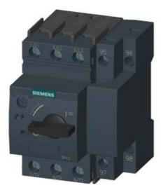
CIRCUIT-BREAKER SZ S00, FOR MOTOR PROTECTION, CLASS 10, W. OVERLOAD RELAY FUNCTION A-RELEASE 0.22...0.32A, N-RELEASE4.2A SCREW CONNECTION, STANDARD SW. CAPACITY
