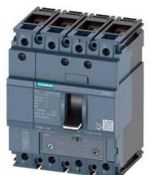
CIRCUIT BREAKER 3VA1 IEC FRAME 160 BREAKING CAPACITY CLASS M ICU=55KA @ 415 V 4-POLE, LINE PROTECTION TM240, ATAM, IN=125A OVERLOAD PROTECTION IR=87,5A ...125A SHORT CIRCUIT PROTECTION II=5...10 X IN NEUTRAL UNPROTECTED BUSBAR CONNECTION
