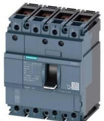
CIRCUIT BREAKER 3VA1 IEC FRAME 160 BREAKING CAPACITY CLASS N ICU=25KA @ 415 V 4-POLE, LINE PROTECTION TM210, FTFM, IN=160A OVERLOAD PROTECTION IR=160A FIXED SHORT CIRCUIT PROTECTION II=10 X IN NEUTRAL PROTECTION 100% BUSBAR CONNECTION
