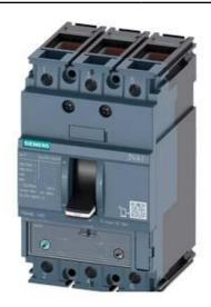
CIRCUIT BREAKER 3VA1 IEC FRAME 160 BREAKING CAPACITY CLASS S ICU=36KA @ 415 V 3-POLE, LINE PROTECTION TM240, ATAM, IN=160A OVERLOAD PROTECTION IR=112A ...160A SHORT CIRCUIT PROTECTION II=5...10 X IN CABLE CONNECTION
