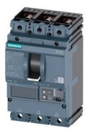
CIRCUIT BREAKER 3VA2 IEC FRAME 100 BREAKING CAPACITY CLASS H ICU=85KA @ 415 V 3POLE, LINE PROTECTION ETU860, LSIG, IN=25A OVERLOAD PROTECTION IR=10A ...25A SHORT CIRCUIT PROTECTION ISD=0,6..10X IN, II=1,5..12X IN NEUTRAL PROTECTION OPTIONAL WITH EXT. CT,UPTO 160% GROUNDFAULT, SWITCHABLE IG=0,2... 1 X IN, TG=0,050,8MS BUSBAR CONNECTION
