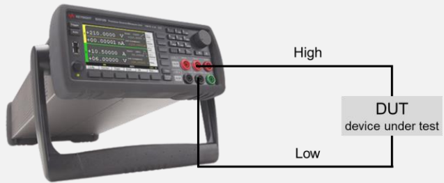
SMU solution: Integrated 4-quadrant voltage and current sourcing and measurement (including AWG function).
