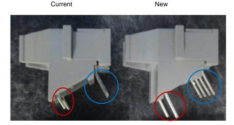
Housing staple pins (pin5 and pin8 in red circle): Length increased from 2.8mm to 4.6mm.
