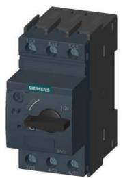
LEISTUNGSSCHALTER BGR. S00, FUER DEN TRAFOSCHUTZ A-AUSL. 2,8...4A, N-AUSL. 82A, SCHRAUBANSCHLUSS, STANDARDSCHALTVERMOEGEN
