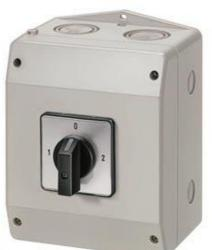
CHANGEOVER SWITCH 3-POLE IU=32, P/AC-23A AT 400V=11,5KW 2 N-TERMINAL MOULDED-PLASTIC ENCLOSURED, IP65
