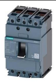
CIRCUIT BREAKER 3VA1 IEC FRAME 160 BREAKING CAPACITY CLASS S ICU=36KA @ 415 V 3-POLE, LINE PROTECTION TM210, FTFM, IN=125A OVERLOAD PROTECTION IR=125A FIXED SHORT CIRCUIT PROTECTION II=10 X IN CABLE CONNECTION
