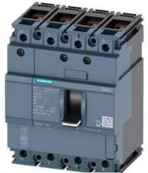
CIRCUIT BREAKER 3VA1 IEC FRAME 160 BREAKING CAPACITY CLASS M ICU=55KA @ 415 V 4-POLE, LINE PROTECTION TM210, FTFM, IN=160A OVERLOAD PROTECTION IR=160A FIXED SHORT CIRCUIT PROTECTION II=10 X IN NEUTRAL PROTECTION 50% BUSBAR CONNECTION
