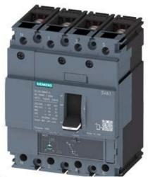
CIRCUIT BREAKER 3VA1 IEC FRAME 160 BREAKING CAPACITY CLASS H ICU=70KA @ 415 V 4-POLE, LINE PROTECTION TM220, ATFM, IN=32A OVERLOAD PROTECTION IR=22,4A ...32A SHORT CIRCUIT PROTECTION II=10 X IN NEUTRAL PROTECTION 100% BUSBAR CONNECTION
