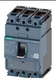
CIRCUIT BREAKER 3VA1 IEC FRAME 160 BREAKING CAPACITY CLASS N ICU=25KA @ 415 V 3-POLE, LINE PROTECTION TM220, ATFM, IN=80A OVERLOAD PROTECTION IR=56A ...80A SHORT CIRCUIT PROTECTION II=10 X IN BUSBAR CONNECTION
