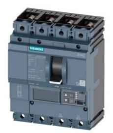
CIRCUIT BREAKER 3VA2 IEC FRAME 160 BREAKING CAPACITY CLASS L ICU=150KA @ 415 V 4POLE, LINE PROTECTION ETU850, LSI, IN=100A OVERLOAD PROTECTION IR=40A ...100A SHORT CIRCUIT PROTECTION ISD=0,6..10X IN, II=1,5..12X IN NEUTRAL PROTECTION ADJUSTABLE (OFF, UPTO 160%) BUSBAR CONNECTION
