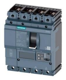
CIRCUIT BREAKER 3VA2 IEC FRAME 160 BREAKING CAPACITY CLASS H ICU=85KA @ 415 V 4POLE, LINE PROTECTION ETU550, LSI, IN=160A OVERLOAD PROTECTION IR=64A ...160A SHORT CIRCUIT PROTECTION ISD=0,6..10X IN, II=1,5..10X IN NEUTRAL PROTECTION ADJUSTABLE (OFF, UPTO 100%) BUSBAR CONNECTION
