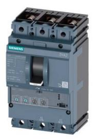
CIRCUIT BREAKER 3VA2 IEC FRAME 160 BREAKING CAPACITY CLASS C ICU=110KA @ 415 V 3POLE, LINE PROTECTION ETU330, LIG, IN=160A OVERLOAD PROTECTION IR=64A ...160A SHORT CIRCUIT PROTECTION II=1,5...10 X IN GROUNDFAULTPROTECTION IG=0,2... 1 X IN, TG=0,1/0,3MS BUSBAR CONNECTION
