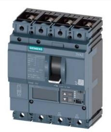
CIRCUIT BREAKER 3VA2 IEC FRAME 250 BREAKING CAPACITY CLASS L ICU=150KA @ 415 V 4POLE, LINE PROTECTION ETU860, LSIG, IN=160A OVERLOAD PROTECTION IR=64A ...160A SHORT CIRCUIT PROTECTION ISD=0,6..10X IN, II=1,5..12X IN NEUTRAL PROTECTION ADJUSTABLE (OFF, UPTO 160%) GROUNDFAULT, SWITCHABLE IG=0,2... 1 X IN, TG=0,050,8MS BUSBAR CONNECTION
