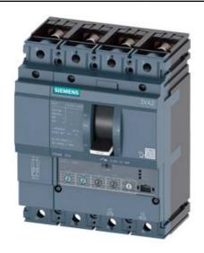
CIRCUIT BREAKER 3VA2 IEC FRAME 250 BREAKING CAPACITY CLASS H ICU=85KA @ 415 V 4POLE, LINE PROTECTION ETU330, LIG, IN=250A OVERLOAD PROTECTION IR=100A ...250A SHORT CIRCUIT PROTECTION II=1,5...10 X IN NEUTRAL PROTECTION ADJUSTABLE(OFF,50%,100%) GROUNDFAULTPROTECTION IG=0,2... 1 X IN, TG=0,1/0,3MS BUSBAR CONNECTION
