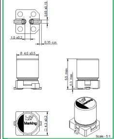
Example new drawings with direct dimensioning
