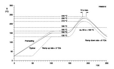
Solid line: Typical process (terminal temperature)
