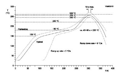
Solid line: Typical process (terminal temperature)
