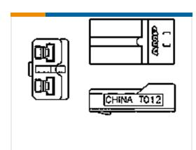
TE Model / Part #521073-2 PLUG .125 HOUSING NYLON 66/6
