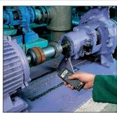
rpm measurement on shafts
