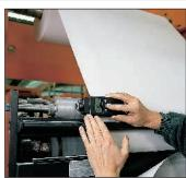
Mechanical rpm measurement on a roller
