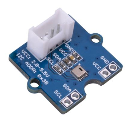
AHT20 is a new generation of temperature and humidity sensor embedded with a dual-row flat and no-lead SMD package, suitable for the reflow soldering. AHT20 is equipped with a newly designed ASIC chip: an improved MEMS semiconductor capacitive humidity sensor, and a standard on-chip temperature sensor. The output is the I2C protocol with the Grove interface.
