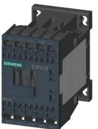
COUPLING CONTACTOR RAIL, AC3:5.5KW,DC110V,0,7...1,25\*US, 1NO, VARISTOR INTEGRATED, 3-POLE, SZ S00 SPRING-LOADED TERMINAL
