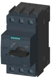
CIRCUIT-BREAKER SZ S0, FOR STARTER COMBINATION, RATED CURRENT 25A, N-RELEASE 325A, SCREW CONNECTION, STANDARD SW. CAPACITY
