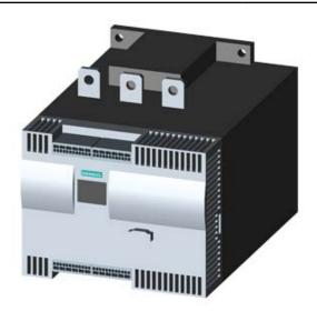
SIRIUS SOFT STARTER, VALUES WITH 690 V, 40 DEG., STANDARD: 203A, 200KW, INSIDE-DELTA CIRCUIT 3: ONLY UP TO 600V, 400-690 V AC, 230 V AC, CAGE CLAMP TERMINALS
