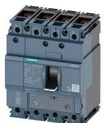
CIRCUIT BREAKER 3VA1 IEC FRAME 160 BREAKING CAPACITY CLASS N ICU=25KA @ 415 V 4-POLE, LINE PROTECTION TM240, ATAM, IN=100A OVERLOAD PROTECTION IR=70A ...100A SHORT CIRCUIT PROTECTION II=5...10 X IN NEUTRAL PROTECTION 50% BUSBAR CONNECTION
