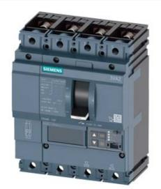
CIRCUIT BREAKER 3VA2 IEC FRAME 100 BREAKING CAPACITY CLASS H ICU=85KA @ 415 V 4POLE, LINE PROTECTION ETU850, LSI, IN=25A OVERLOAD PROTECTION IR=10A ...25A SHORT CIRCUIT PROTECTION ISD=0,6..10X IN, II=1,5..12X IN NEUTRAL PROTECTION ADJUSTABLE (OFF, UPTO 160%) BUSBAR CONNECTION
