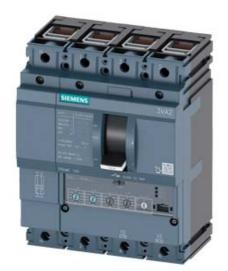
CIRCUIT BREAKER 3VA2 IEC FRAME 160 BREAKING CAPACITY CLASS M ICU=55KA @ 415 V 4POLE, LINE PROTECTION ETU350, LSI, IN=100A OVERLOAD PROTECTION IR=40A ...100A SHORT CIRCUIT PROTECTION ISD=1,5... 10 X IR, II=12 X IN NEUTRAL PROTECTION ADJUSTABLE(OFF,50%,100%) CABLE CONNECTION
