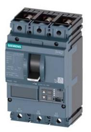
CIRCUIT BREAKER 3VA2 IEC FRAME 160 BREAKING CAPACITY CLASS M ICU=55KA @ 415 V 3POLE, LINE PROTECTION ETU560, LSIG, IN=100A OVERLOAD PROTECTION IR=40A ...100A SHORT CIRCUIT PROTECTION ISD=0,6..10X IN, II=1,5..12X IN NEUTRAL PROTECTION OPTIONAL WITH EXT. CT,UPTO 160% GROUNDFAULT, SWITCHABLE IG=0,2... 1 X IN, TG=0,050,8MS BUSBAR CONNECTION
