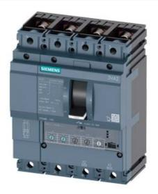
CIRCUIT BREAKER 3VA2 IEC FRAME 160 BREAKING CAPACITY CLASS H ICU=85KA @ 415 V 4POLE, LINE PROTECTION ETU350, LSI, IN=160A OVERLOAD PROTECTION IR=64A ...160A SHORT CIRCUIT PROTECTION ISD=1,5... 10 X IR, II=10 X IN NEUTRAL PROTECTION ADJUSTABLE(OFF,50%,100%) BUSBAR CONNECTION
