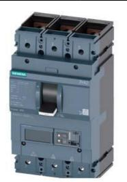
CIRCUIT BREAKER 3VA2 IEC FRAME 400 BREAKING CAPACITY CLASS M ICU=55KA @ 415 V 3-POLE, LINE PROTECTION ETU860, LSIG, IN=250A OVERLOAD PROTECTION IR=100A ...250A SHORT CIRCUIT PROTECTION ISD=0,6..10X IN, II=1,5..12X IN NEUTRAL PROTECTION OPTIONAL WITH EXT. CT;UPTO 160% GROUND-FAULT, SWITCHABLE IG=0,2... 1 X IN, TG=0,05-0,8MS BUSBAR CONNECTION
