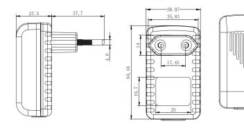
Dimensions : Millimetres Tolerance : ± 0.2mm
