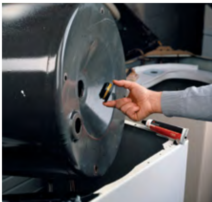
Immediately bond and seal: 3M™ Nitrile High Performance Rubber and Gasket Adhesive 847 (pg 19)
