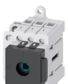
Switch disconnector 3LD3, main switch 3-polig, lu 32A operational switch at AC-23 A at 400 V 11,5 kW Distribution board mounting Base mounting without knob-operated mechanism with auxiliary 1NO+1NC
