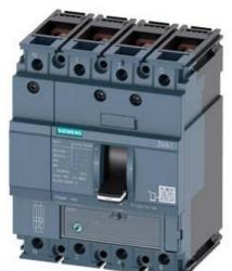
CIRCUIT BREAKER 3VA1 IEC FRAME 160 BREAKING CAPACITY CLASS S ICU=36KA @ 415 V 4-POLE, LINE PROTECTION TM220, ATFM, IN=100A OVERLOAD PROTECTION IR=70A ...100A SHORT CIRCUIT PROTECTION II=10 X IN NEUTRAL UNPROTECTED BUSBAR CONNECTION
