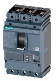
CIRCUIT BREAKER 3VA2 IEC FRAME 160 BREAKING CAPACITY CLASS C ICU=110KA @ 415 V 3POLE, LINE PROTECTION ETU560, LSIG, IN=160A OVERLOAD PROTECTION IR=64A ...160A SHORT CIRCUIT PROTECTION ISD=0,6..10X IN, II=1,5..10X IN NEUTRAL PROTECTION OPTIONAL WITH EXT. CT,UPTO 160% GROUNDFAULT, SWITCHABLE IG=0,2... 1 X IN, TG=0,050,8MS BUSBAR CONNECTION
