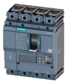
CIRCUIT BREAKER 3VA2 IEC FRAME 160 BREAKING CAPACITY CLASS L ICU=150KA @ 415 V 4POLE, LINE PROTECTION ETU550, LSI, IN=160A OVERLOAD PROTECTION IR=64A ...160A SHORT CIRCUIT PROTECTION ISD=0,6..10X IN, II=1,5..10X IN NEUTRAL PROTECTION ADJUSTABLE (OFF, UPTO 100%) CABLE CONNECTION
